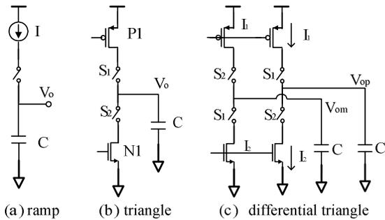
Fig.1. Capacitor charging circuits
