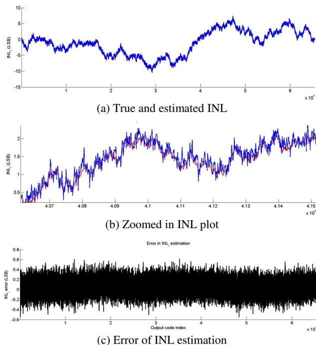
Fig.5. INL estimation error for 16 bit ADC
