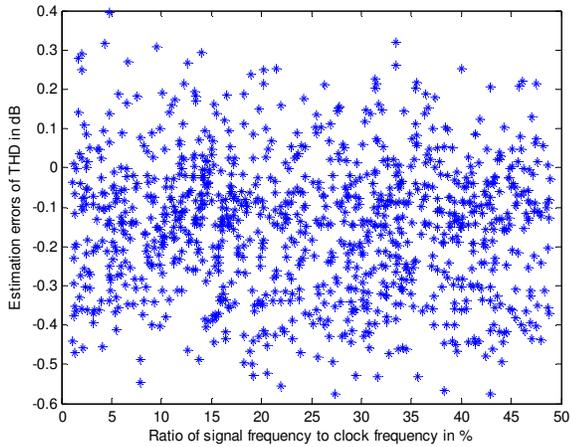
Figure 11 THD testing errors in 1000 runs using the proposed method, vs  $f_{in}/f_s * 100$
