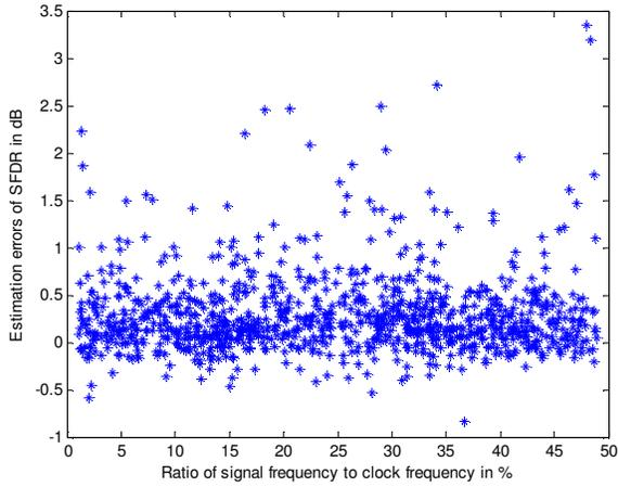
Figure 10 SFDR testing errors in 1000 runs using the proposed method, vs  $f_{in}/f_s * 100$
