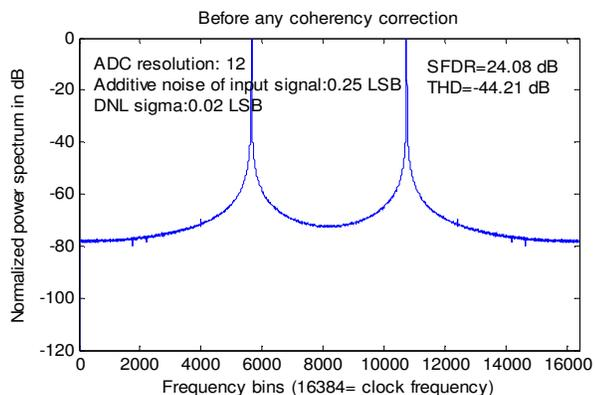
Figure 2 Straightforward application DFT to the noncoherent data samples
