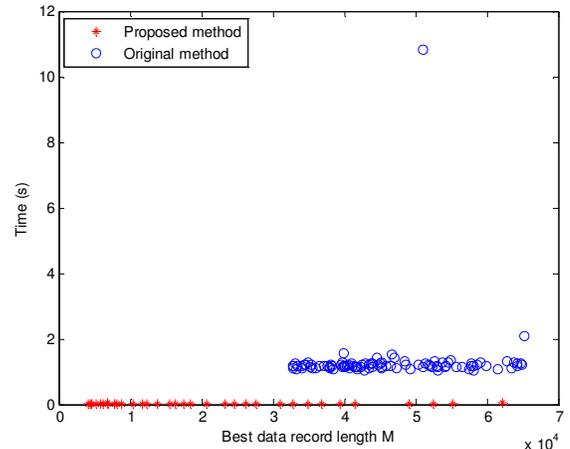
Figure 12 Time in 100 runs using the proposed method and original method respectively, vs the best data record M
