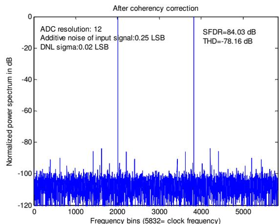
Figure 3 Spectrum of the noncoherent data samples using the proposed method
