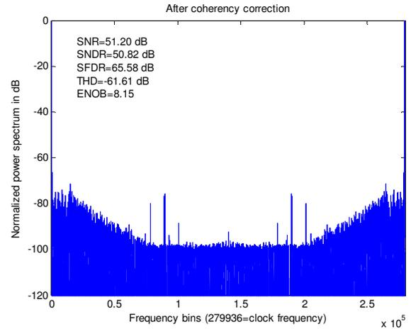
Figure 8 Spectrum of the noncoherent data samples using the proposed method
