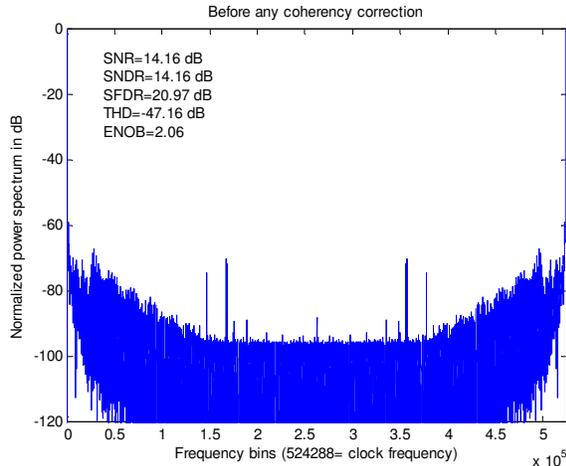
Figure 6 Spectrum by standard application of DFT Before any coherency correction
