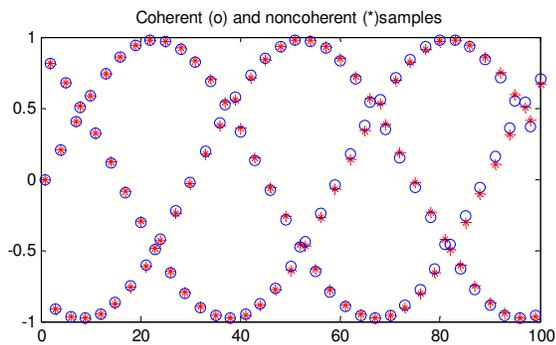
Figure 1 Data samples from coherent and noncoherent sampling
