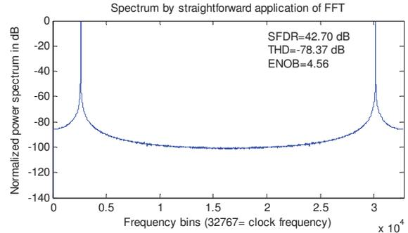
Fig. 6 Straightforward application of FFT to the noncoherent data samples
