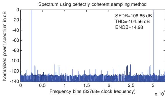
Fig. 11 Spectrum obtained by the perfectly coherent sampling method
