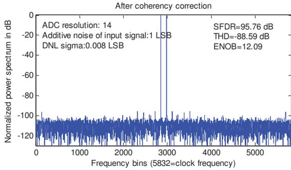
Fig. 3 Spectrum of the noncoherent data samples using the proposed method
