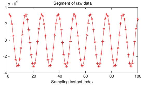
Fig. 5 Time domain data samples from the noncoherent sampling
