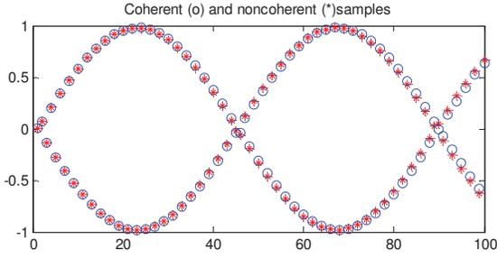
Fig. 1 Data samples from coherent and noncoherent sampling
