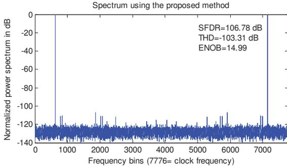
Fig. 9 Spectrum obtained by the proposed method
