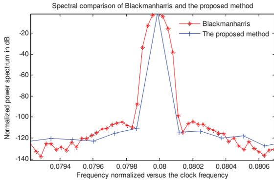
Fig. 10 Spectral comparison of Blackmanharris method and the proposed method around the signal bin
