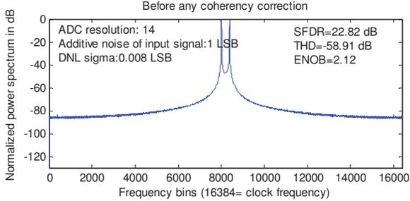
Fig. 2 Straightforward application FFT to the noncoherent data samples
