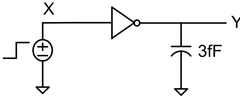
$$t_{HL} \cong R_{SWn} C_L = 2K \bullet 3fF = 6p \text{ sec}$$
