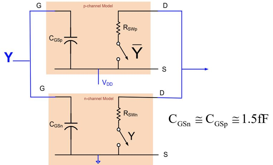
Loading effects same whether  $C_{GSp}$  and/or  $C_{GSn}$  connected to  $V_{DD}$  or GND
